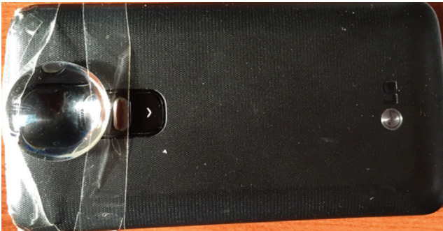
Figure 1. A 90 Diopter non-contact double aspheric lens was attached to the posterior camera of a smartphone using clear tape
