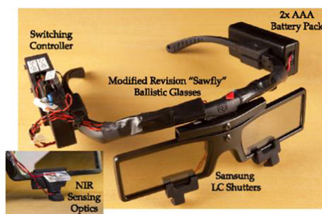
Figure 7. The glasses worn with telescopic scleral contact lenses
