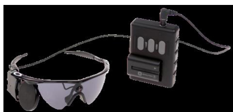
Figure 8. Argus II, extraocular part ( http://second sight.com/photos.html . Accessed on 08.18.2018)
