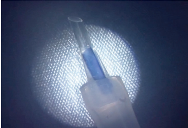
Figure 2. The tip of an IOL injector cartridge was combined with a silicone tubing set to create the custom-made injector
